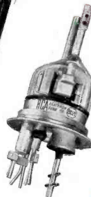
RCA-8D21 used in 5-kw television transmitters
